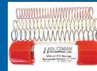
Holtzman Engineering's new "altitude specific" springs for the Yamaha RX-1's CV carbs promise to keep the big four-stroke from losing too much power as you gain elevation. Three different springs are available: green for up to 4,000 feet; yellow for 4,000-8,000; and red for 8,000-12,000. The springs are easy to install and come in a convenient storage tube. Cost is \$34 (US) for a set of four; more info from [www.holtzmaneng.com](http://www.holtzmaneng.com), or call (715) 479-8727.
